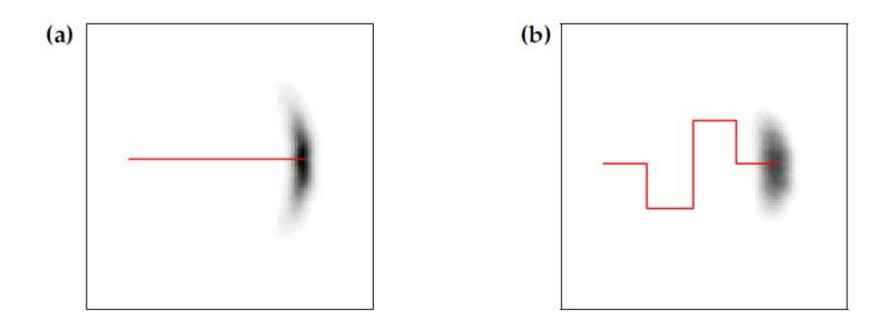
**Figure 5.2** The motion model: Posterior distributions of the robot's pose upon executing the motion command illustrated by the solid line. The darker a location, the more likely it is. This plot has been projected into 2-D. The original density is three-dimensional, taking the robot's heading direction  $\theta$  into account.
